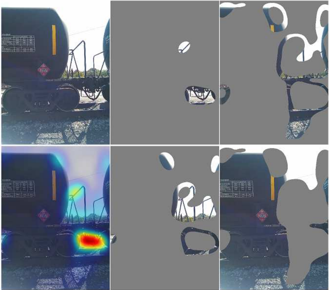
Fig. 3.25. An example of lost saliency map with the four types of salient regions (top to bottom then left to right): original image, lost saliency map; high salient regions, middle salient regions; low salient regions, non-salient regions.
