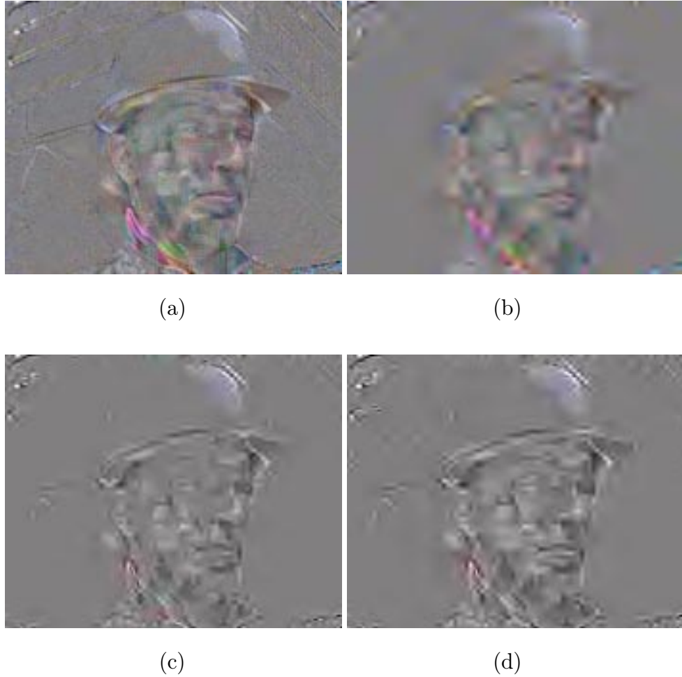
Fig. 4.31. Experiment #3: (a) PEF from frame 35 of the foreman sequence. (b) PEF in (a) encoded using CEZW and decoded at 0.25 bpp. (c) PEF in (a) after preprocessing, modified CEZW , and postprocessing. (d) PEF in (a) encoded using CEZW+ and decoded at 0.25 bpp.
