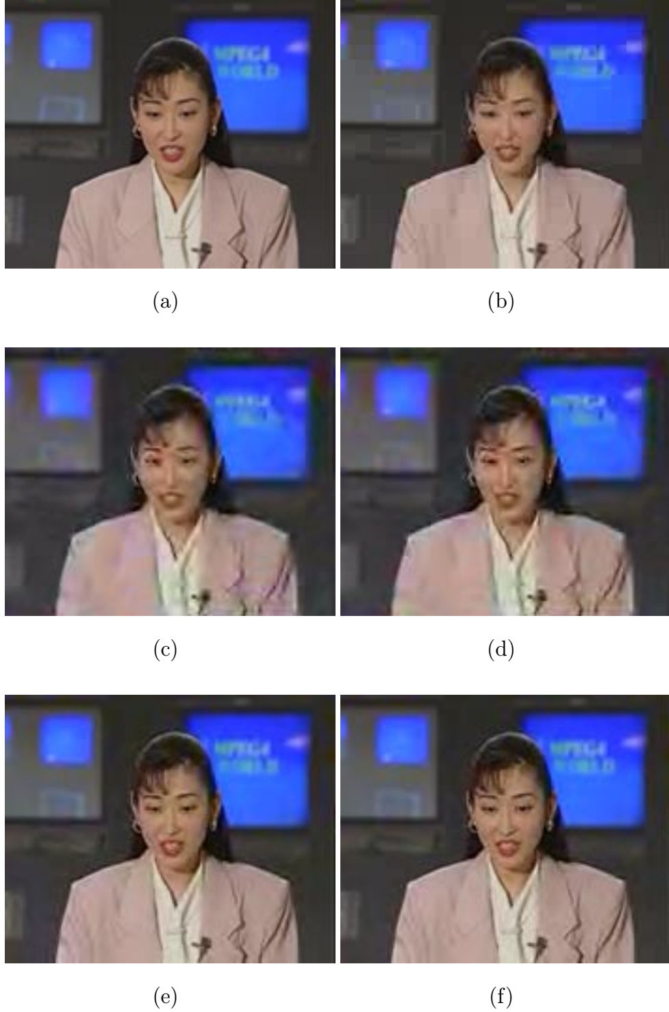
Fig. 4.41. Comparison of Experiments #1, #2, and #3: Decoded frames of the akiyo sequence at 16 kbps, 5 fps. (a) Original. (b) H.263+. (c) SAMCoW . (d) SAMCoW : AVCT. (e) SAMCoW : PP. (f) SAMCoW+ .
