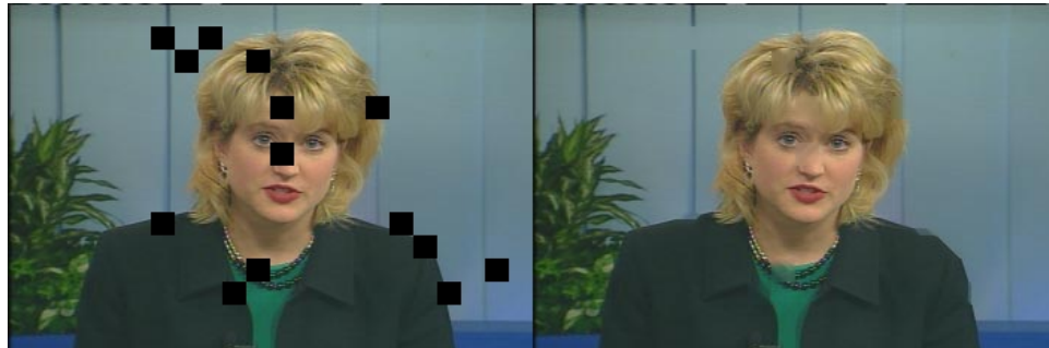
Fig. 2.27. Frame from an MPEG sequence with missing macroblocks before and after error concealment.
