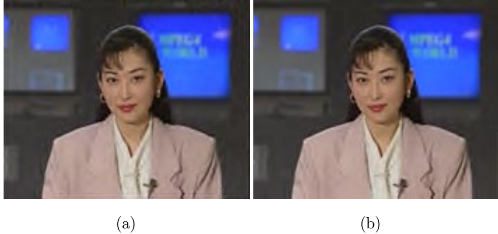
Fig. 2.23. Comparison between periodic and whole-sample symmetric extension when used within an image compression scheme. Artifacts near the bottom boundary of the image are noticeable when using (a) periodic instead of (b) whole-sample symmetric (WSS) extension.
