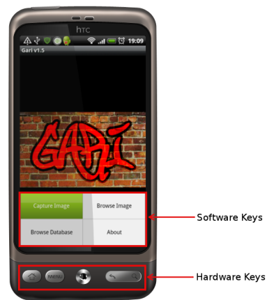
Fig. 3.6.: Difference Between Hardware and Software Keys on the HTC Desire Mobile Telephone.
