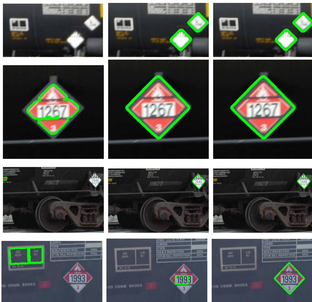
Fig. 5.38.: Examples of sign location detection. Column from left to right: results from [257], results from [314], results from proposed method.
