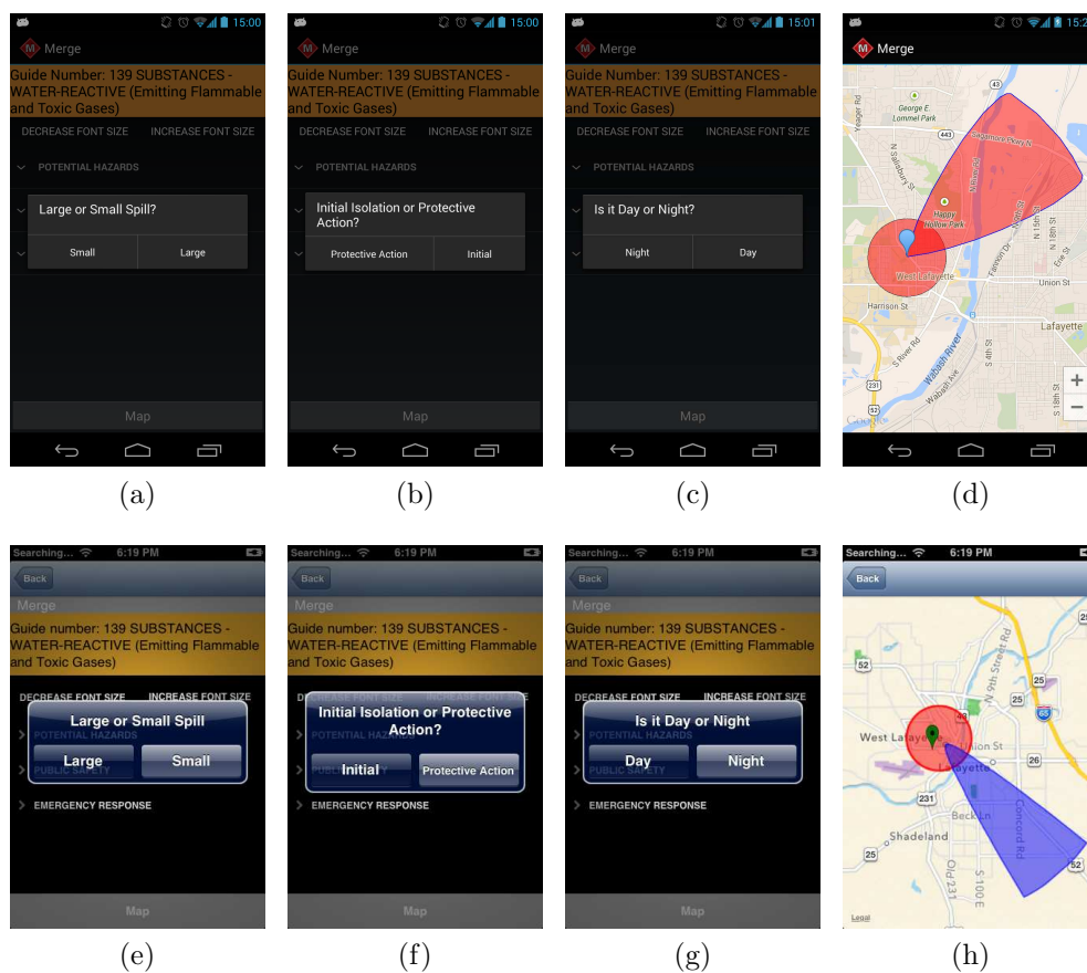
Fig. 4.30.: Evacuation region for Android (top) and iPhone (bottom). From left to right, questions asked to refine evacuation region, and general evacuation circle and weather-based plume model.
