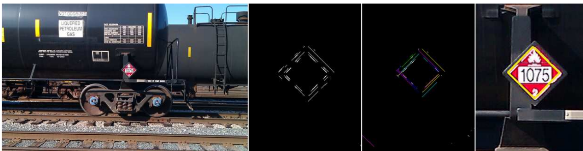
Fig. 4.3.: First method (left to right): original image, segments at \pm 45^\circ , grouped segments, optimal bounding box.
