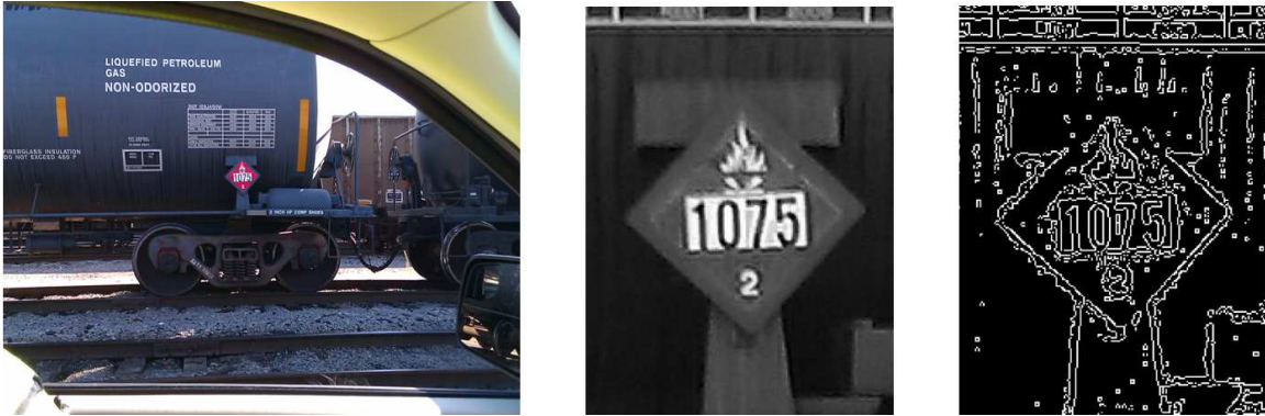
Fig. 4.4.: Issue With First Method: Grayscale. Sign Is Lost On Line Detection Process.
