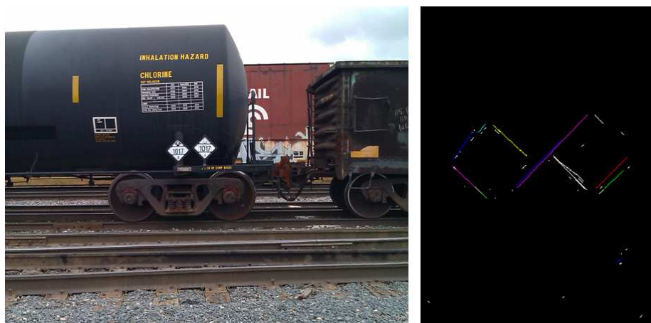
Fig. 4.7.: Issue With First Method: Segment Merging. Sign Is Lost On Segment Grouping Process.
