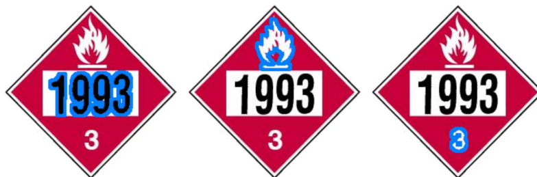
Fig. 2.9.: Elements That Uniquely Identify a Hazmat Sign. From Left to Right: UNID, Symbol, and Class Number.
