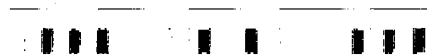
■ Figure 4. Position of the resynchronization markers in the bitstream for a baseline H.263 encoder with GOB headers.
