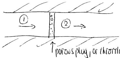
Steady flowthrough a hear-insularing pipe with a porous plug.
