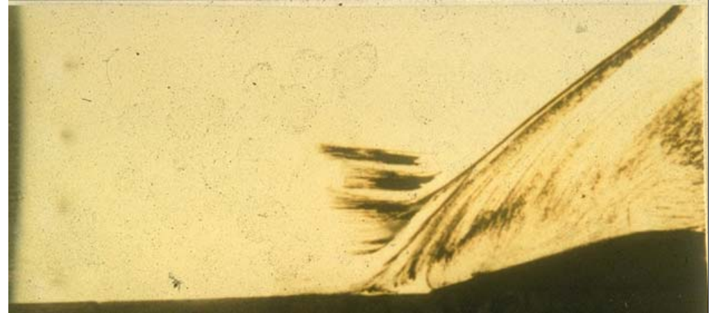
Oil Flow on Side Wall
