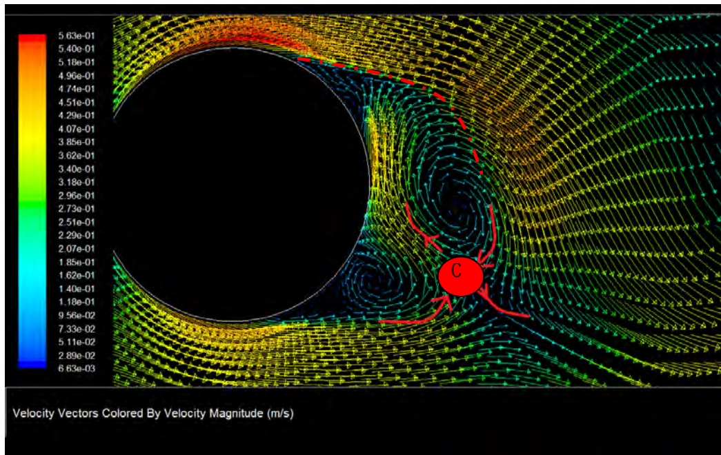
Figure 22: Instantaneous magnified image of the simulated flow domain indicating the presence of the confluence point in the wake after 260 time steps
