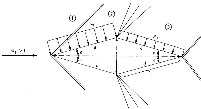
Figure 1: Double-Wedge Geometry (from Anderson, Fundamentals, 4e)
