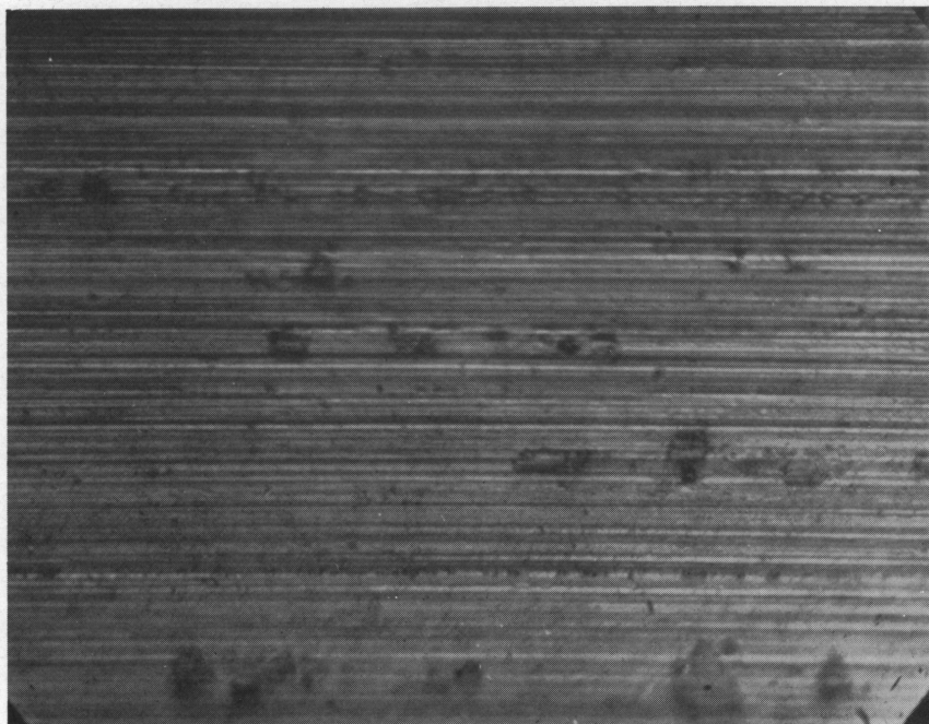
(a) Longitudinal scratches on the cylinder; X400.
