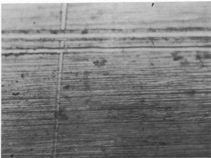
Figure 4.- Grooves produced by profilometer stylus on an emery-polished model; X400.
