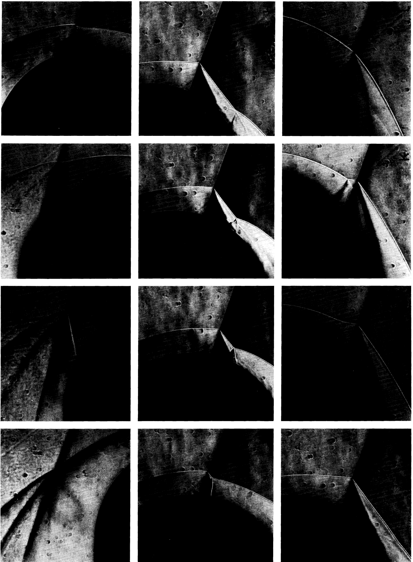
Fig. 6.1. Interference patterns on hemisphere. M = 4.6 , \xi = 5^\circ .
