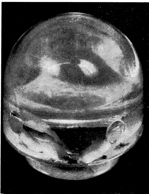
Fig. A.1. Hemispherical glass model prior to application of gauges and leads.
