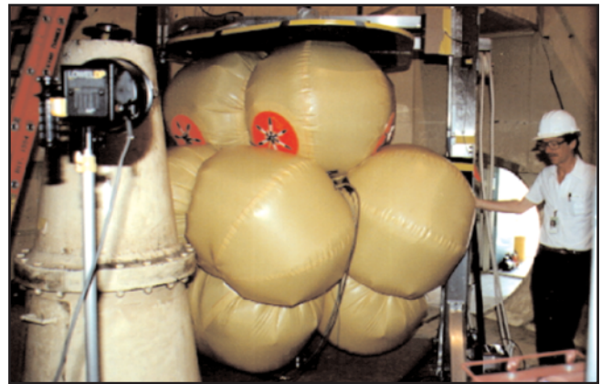
Airbag configurations mounted in the High-Altitude Chamber for impact testing as part of Sandia's work for NASA and JPL for the Pathfinder surface landing missions on Mars.
