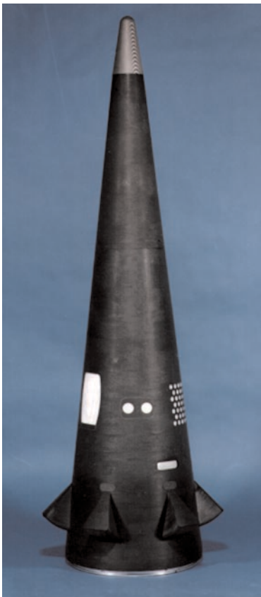
The IRV-2 vehicle (left) was a U.S. Air Force-sponsored reentry vehicle flown in support of the Maneuvering Systems Technology (MaST) Program. Recently, coupled fluid/thermal ablations calculations have been performed on geometries similar to the IRV-2 vehicle to simulate the ablation characteristics of thermal protection systems. Simulations of the carbon-carbon nosetip show the amount of surface recession and mesh deformation of both the fluid (blue) and thermal (red) meshes on representative trajectories.
