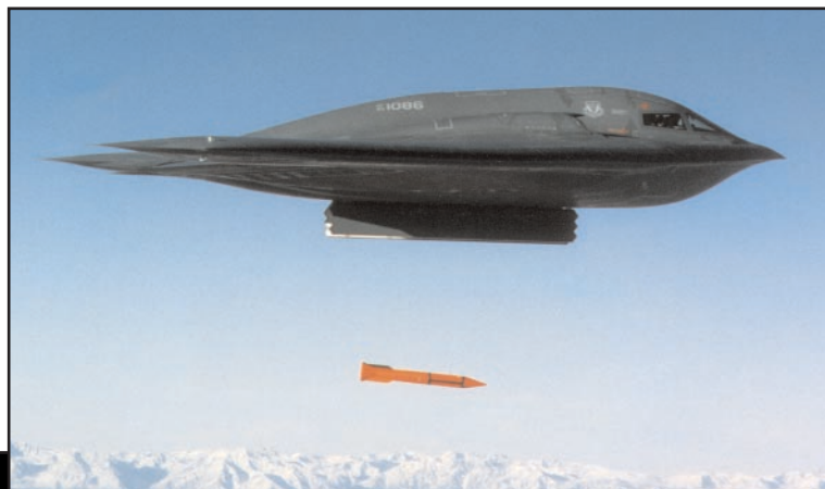
The B61-11 in flight with spin rockets firing. Code predictions using Full Navier-Stokes calculations are used in concert with flight and ground testing to understand interactions between the spin rocket plumes and the fins.
