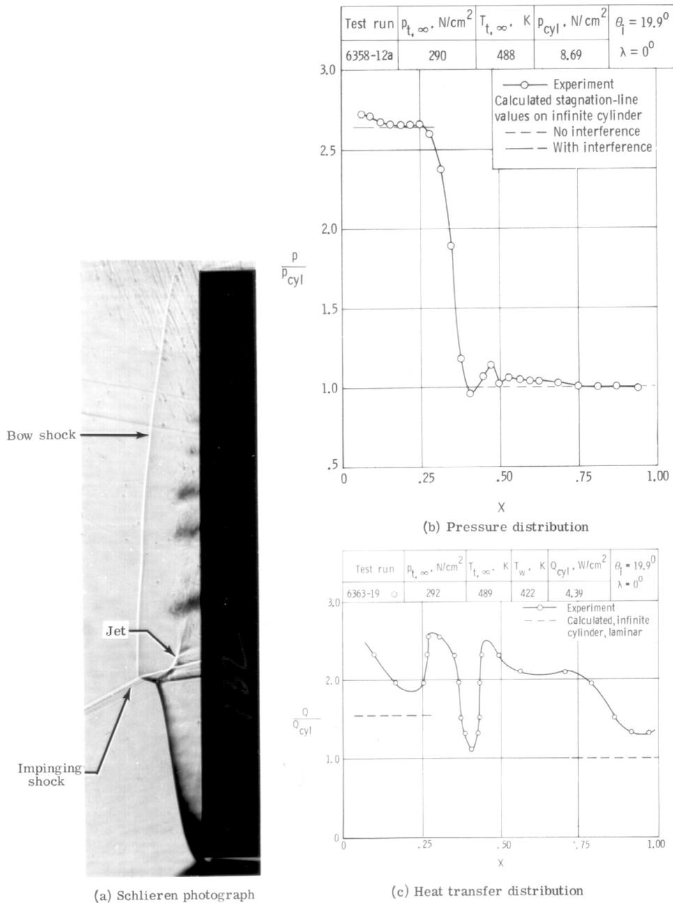
Figure I-27.- Type IVa interference on a fin at Mach 6 in air.
