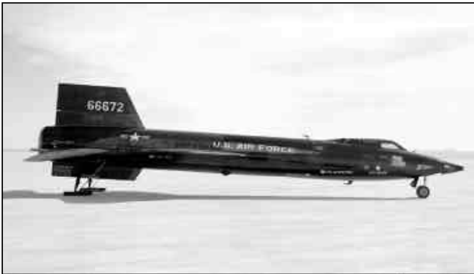
The X-15 ship Number 3 (56-6672) is seen here on the lakebed at the Edwards Air Force Base, California. Ship Number 3 made 65 flights during the program, attaining a top speed of Mach 5.65 and a maximum altitude of 354,200 feet. (NASA photo E-7896)
