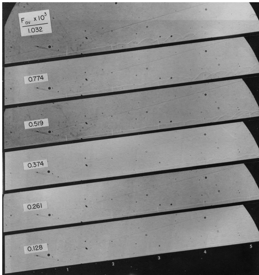
Fig. 3 Shadowgraph of instabilities with helium blown into air, from figure 3d in [12].
