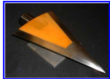
Figure 9a. Temperature Sensitive Paint on HTV-2 Forebody Tested in Purdue Quiet Flow Ludwig Tube 48
