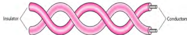
Figure 11.2: A twisted pair transmission line where the two wires are not parallel to each other (courtesy of slides by A. Wadhwa, A.L. Dal, N. Malhotra [90].)
