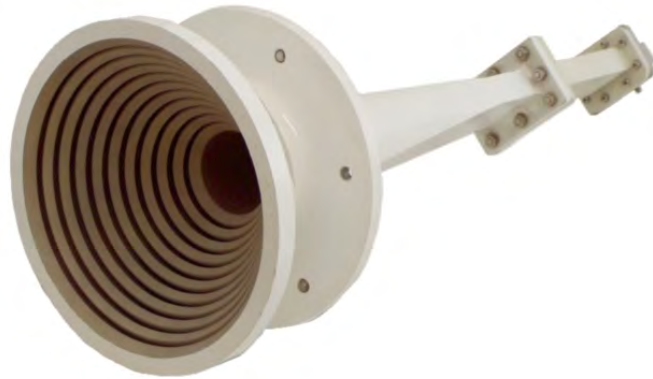
Figure 20.5: Picture of a circular horn antenna where corrugated wall is used to enhance the TE_{01} mode and discourage the other modes (courtesy of [135]).
