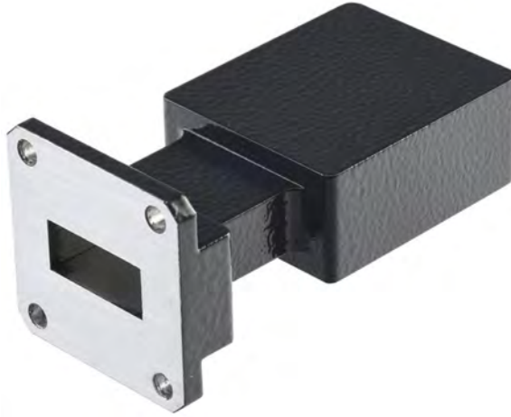
Figure 21.3: A rectangular waveguide terminated with a short at one end, and an open circuit at the other end. The open end can also act as an antenna as it also radiates. When the cavity is injected with electromagnetic fields coinciding with its resonance frequency, the fields inside the cavity becomes large, so does the fields at the aperture, making it a better radiator. This is a cavity-backed antenna: it uses resonance tunneling to enhance its radiation capability (courtesy of RFcurrent.com).
