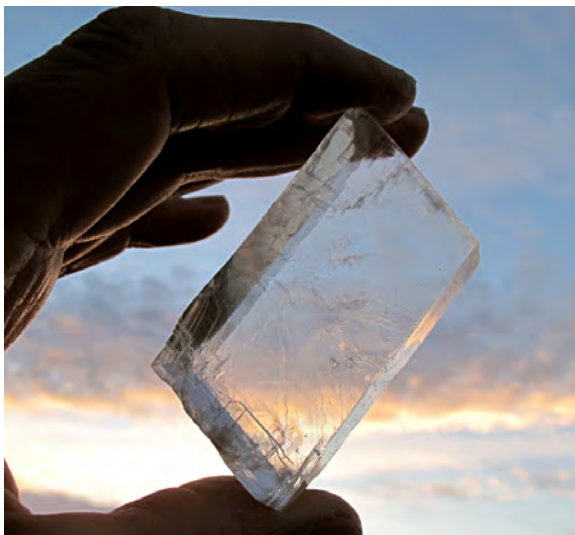
Figure 34.4: A sunstone can indicate the polarization of the scattered light. From that, one can deduce where the sun is located (courtesy of Wikipedia).
