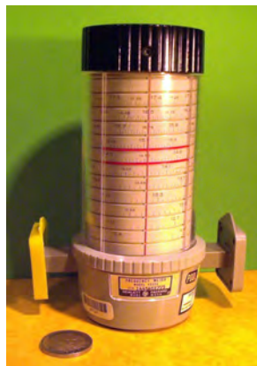
Figure 21.15: An absorption wave meter can be used to measure the frequency of microwave. If the microwave energy enters the cavity at its resonant frequency, strong field buildup inside the cavity causes increased loss and absorption of the microwave energy by the cavity. A dip in energy level of the transmitted signal indicated the coincidence of the resonant frequency of the microwave with the frequency of the microwave (courtesy of Wiki [143]).
