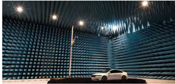
Figure 37.5: An anechoic chamber for radio frequency. In such an electromagnetically quiet chamber, interference from other RF equipment is minimized (courtesy of Panasonic).
