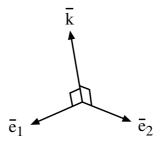
**Figure 1.3.4** The electric field vectors and the **k** vector in an isotropic medium.
