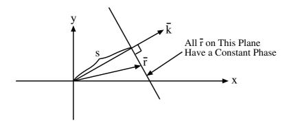
Figure 1.2.1 Constant phase front of a plane wave which is perpendicular to k.
