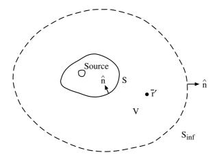
Figure 1.4.1 The geometry for the derivation of Huygens' principle.
