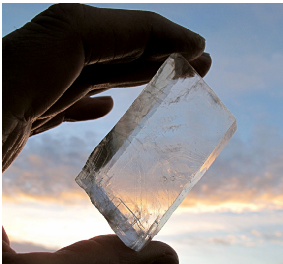
Figure 34.4: A sunstone can indicate the polarization of the scattered light. From that, one can deduce where the sun is located; either behind us or in front of us (courtesy of Wikipedia).
