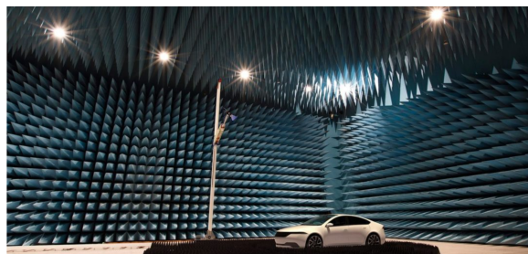
Figure 37.6: An anechoic chamber for radio frequency. In such an electromagnetically quiet chamber, interference from other RF equipment is minimized (courtesy of Panasonic).
