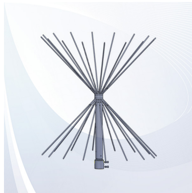
Figure 28.11: A bicone antenna can be thought of as a flared transmission line with gradually changing characteristic impedance. This enhances impedance matching and the radiation of the antenna (courtesy of antennasproduct.com).
