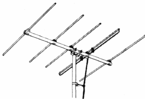
Figure 31.3: A Yagi-Uda antenna was invented by heuristics and great physical insight in 1926 even before we had computers. The principal element of the antenna is the folded dipole with four times the radiation resistance of a half-wave dipole. When an array of wire dipole antenna, each of which is less than half a wavelength, the array acts as a waveguide, or a director. When the wire antenna is slightly more than half a wavelength, the wire dipole ceases to be a waveguide, and it acts as a reflector [202]. Therefore, the antenna radiates predominantly in one direction (courtesy of Wikipedia [203]).
