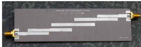
Figure 25.11: A microstrip filter designed using concatenated resonators. The connectors to the coax cable are the SMA (sub-miniature type A) connectors (courtesy of aginas.fe.up.pt).
