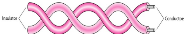
Figure 15.2: A twisted pair transmission line where the two wires are not parallel to each other (courtesy of slides by A. Wadhwa, A.L. Dal, N. Malhotra [122]). The winding of the wires in series opposition cancels the linkage of the transmission line to low frequency external magnetic flux.
