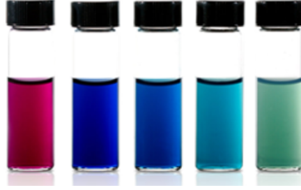
Figure 27.5: Different color fluids containing nano-particles can be obtained by changing the permittivity \varepsilon of the background fluids in (27.3.6) and (27.3.7) (courtesy of nanocomposix.com).
