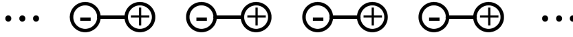
Figure 7.1: As a series of dipoles lined up end to end, one can see a current, through capacitive coupling, flowing through the line of dipoles as they oscillate back and forth in their polarity. This is similar to how displacement current flows through a series of capacitors.
