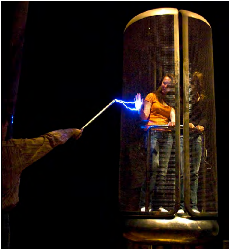
Figure 32.4: Faraday cage demonstration on volunteers in the Palais de la Découverte in Paris (courtesy of Wikipedia). When the cage is grounded, the potential at the surface of the cage is zero. By the solution to Laplace's equation, the potential inside the cage is a constant. Hence, the electric field inside the cage is zero. Charges will surge from the ground to the cage surface to ensure zero potential inside the cage. Therefore, a grounded Faraday cage effectively shields the external fields from entering the cage.
