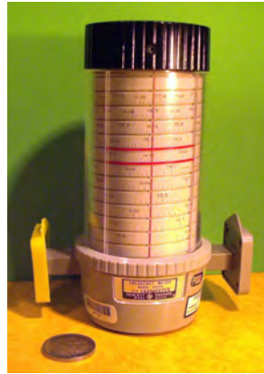
Figure 25.17: An absorption wave meter can be used to measure the frequency of microwave. If the microwave energy enters the cavity at its resonant frequency, strong field buildup inside the cavity causes increased loss and absorption of the microwave energy by the cavity. A dip in energy level of the transmitted signal indicates the coincidence of the resonant frequency of the microwave with the frequency of the passing microwave (courtesy of Wiki [178]).
