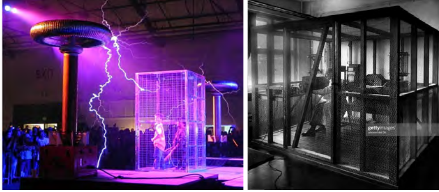
Figure 5.5: (Left) The Faraday cage can be used to shield out low-frequency electromagnetic fields using charges on the surface of the cage, e.g., it is immune to lightning strike (courtesy of defendershield.com). (Right) It can be used to establish an electromagnetically quiet zone free from RF signals (courtesy of Wikipedia).
