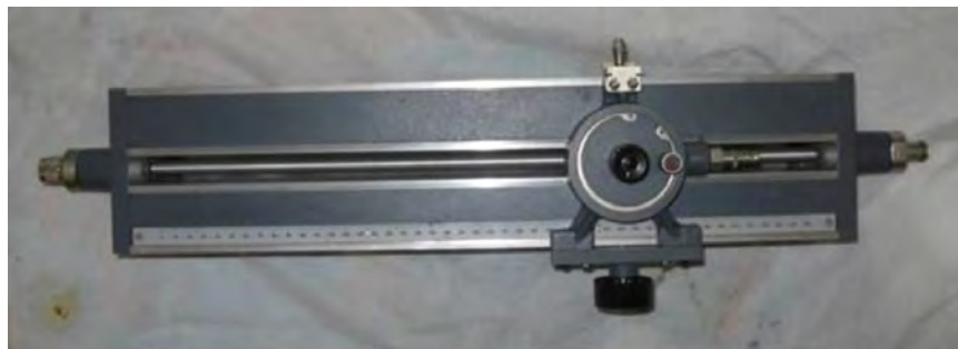
Figure 16.7: A slotted-line equipment which consists of a coaxial waveguide with a slot opening at the top to allow the measurement of the field strength, and hence, the voltage standing wave pattern in the waveguide (courtesy of Microwave101.com).
