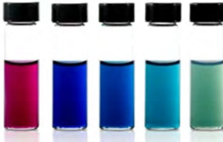
Figure 8.7: Nanoparticles immersed in different solutions will reflect light of different colors (courtesy of nanocomposix.com).
