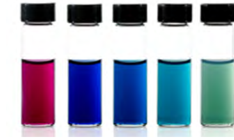
Figure 27.5: Different color fluids containing nano-particles can be obtained by changing the permittivity \varepsilon of the background fluids in (27.3.6) and (27.3.7) (courtesy of nanocomposix.com).
