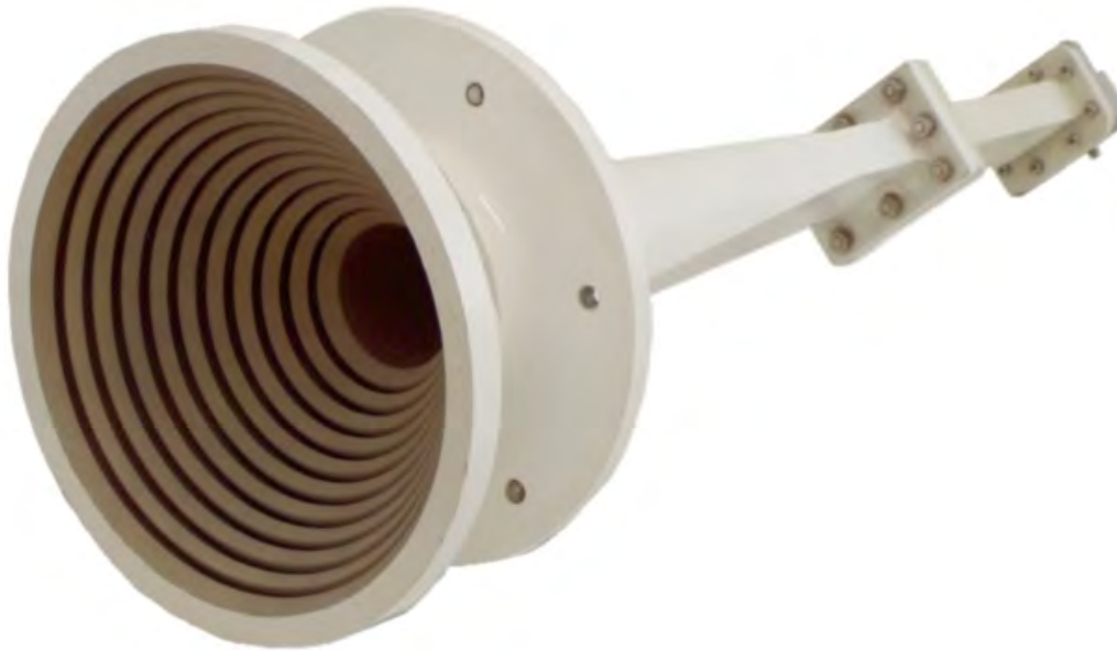
Figure 24.5: Picture of a circular horn antenna where corrugated wall is used to enhance the TE_{01} mode that is axially symmetric. It discourages the other nonaxially symmetric modes. Therefore, the antenna has an axially symmetric field producing a radiation pattern (to be addressed later) that is axially symmetric (courtesy of [170]).
