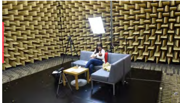
Figure 37.7: An acoustic anechoic chamber. In such a chamber, there is no reflection from the walls of the chamber; even the breast-feeding sound of a baby can be heard clearly (courtesy of AGH University, Poland).
