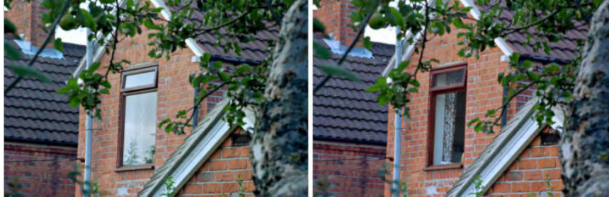
Figure 19.3: Because that TM and TE lights will be reflected differently, polarizer filter can produce remarkable effects on the quality of the photograph by reducing glare [148].
