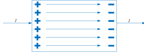
Figure 14.3: The schematic of the field inside a resistor. Due to charge accumulation, the potential on the left side is always higher than that on the right side. An electric field thus points from the left to the right inside the resistor.
