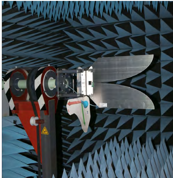
Figure 31.7: A Vivaldi antenna, also called a notched antenna, works like a horn antenna, but uses very little metal and is lightweight. Hence, it is cheap to build, and its flared notch makes it broadband. It is broadband because the high frequency signals can radiate from the narrow part of the notch, and the lower frequency signals can radiate from the wider part of the notch (courtesy of Wikipedia [194]).
