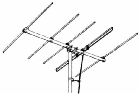
Figure 31.3: A Yagi-Uda antenna was invented by heuristics in 1926. The principal element of the antenna is the folded dipole with four times the radiation resistance of a half-wave dipole. When a wire dipole antenna is less than half a wavelength, it acts as a waveguide, or a director. When the wire antenna is slightly more than half a wavelength, it acts as a reflector [185]. Therefore, the antenna radiates predominantly in one direction (courtesy of Wikipedia [186]).
