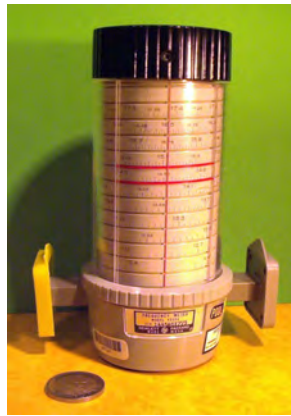
Figure 25.16: An absorption wave meter can be used to measure the frequency of microwave. If the microwave energy enters the cavity at its resonant frequency, strong field buildup inside the cavity causes increased loss and absorption of the microwave energy by the cavity. A dip in energy level of the transmitted signal indicates the coincidence of the resonant frequency of the microwave with the frequency of the microwave (courtesy of Wiki [166]).
