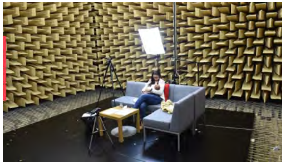
Figure 37.6: An acoustic anechoic chamber. In such a chamber, there is no reflection from the wall of the chamber; even the breast-feeding sound of a baby can be heard clearly (courtesy of AGH University, Poland).
