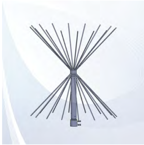
Figure 28.12: A bicone antenna can be thought of as a transmission line with gradually changing characteristic impedance. This enhances impedance matching and the radiation of the antenna (courtesy of antennasproduct.com ).
