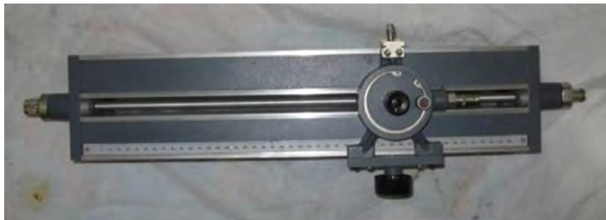
Figure 16.8: A slotted-line equipment which consists of a coaxial waveguide with a slot opening at the top to allow the measurement of the field strength and hence, the voltage standing wave pattern in the waveguide (courtesy of Microwave101.com).
