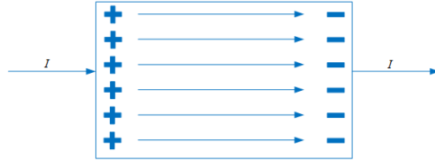
Figure 14.2: The schematic of the field inside a resistor. Due to charge accumulation, the potential on the left side is always higher than that on the right side. An electric field thus points from the left to the right inside the resistor.
