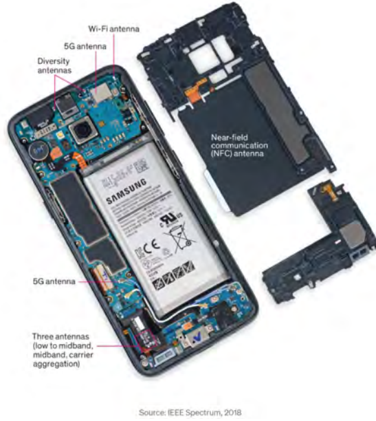
Figure 32.1: The compact locations of the cell phone components make urgent use of EMC/EMI knowledge instrumental in the design of cell phones. Clever use of shielding is necessary to prevent interferences between different components. Compatibility means that even when each component works well in isolation, but when brought to work together, they failed.
