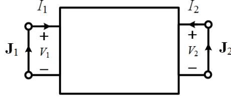
Figure 12.6: The interaction between two antennas in the far field of each other can be reduced to a circuit theory description since the input and output ports of the antennas are small compared to wavelength.
