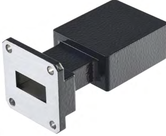
Figure 25.4: A rectangular waveguide terminated with a short at one end, and an open circuit at the other end. The open end can also act as an antenna as it also radiates. When the cavity is injected with electromagnetic fields coinciding with its resonance frequency, the fields inside the cavity becomes large, so does the fields at the aperture, making it a better radiator. This is a cavity-backed antenna: it uses resonance tunneling to enhance its radiation capability (courtesy of RFcurrent.com).
