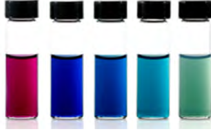
Figure 27.5: Different color fluids containing nano-particles can be obtained by changing the permittivity \varepsilon of the background fluids in (27.3.25) and (27.3.26) (courtesy of nanocomposix.com).
