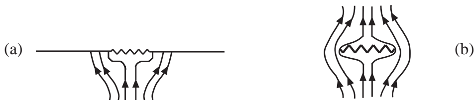
Figure 4.26: Equivalent problem of the \mathbf{E} field around a waveguide wall partially covered by a small magnetic wall.
