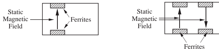
Figure 3.26: Ferrite loading for resonance isolators.
