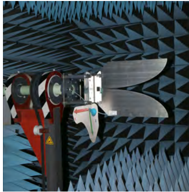
Figure 28.7: A Vivaldi antenna, also called a notch antenna, works like a horn antenna, but uses very little metal. Hence, it is cheap to build, and its flared notch makes it broadband (courtesy of Wikipedia [156]).
