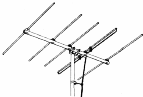
Figure 28.3: A Yagi-Uda antenna was invented by heuristics in 1926. The principal element of the antenna is the folded dipole. When a wire dipole antenna is less than half a wavelength, it acts as a waveguide, or a director. When the wire antenna is slightly more than half a wavelength, it acts as a reflector [148]. Therefore, the antenna radiates predominantly in one direction (courtesy of Wikipedia [149]).
