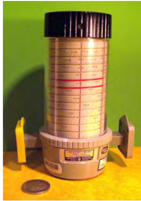
Figure 21.15: An absorption wave meter can be used to measure the frequency of microwave (courtesy of Wiki [130]).
