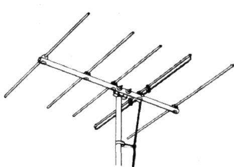
Figure 28.3: A Yagi-Uda antenna was invented by heuristics in 1926. The principal element of the antenna is the folded dipole. When a wire dipole antenna is less than half a wavelength, it acts as a waveguide, or a director. When the wire antenna is slightly more than half a wavelength, it acts as a reflector [148]. Therefore, the antenna radiates predominantly in one direction (courtesy of Wikipedia [149]).
