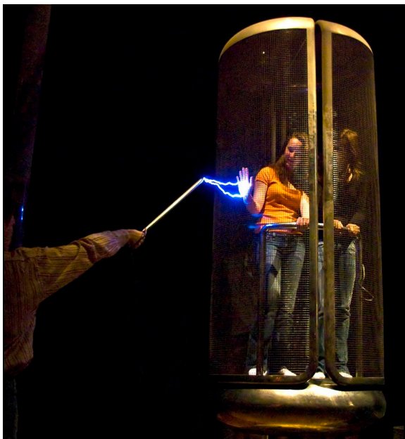
Figure 32.3: Faraday cage demonstration on volunteers in the Palais de la Découverte in Paris (courtesy of Wikipedia). When the cage is grounded, charges will surge from the ground to the cage surface so as to make the field inside the cage zero, or the potential is constant. Therefore, a grounded Faraday cage effectively shields the external fields from entering the cage.
