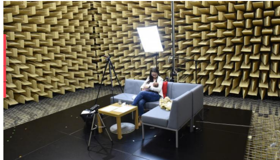
Figure 37.6: An acoustic anechoic chamber. In such a chamber, even the breast-feeding sound of a baby can be heard clearly (courtesy of AGH University, Poland).
