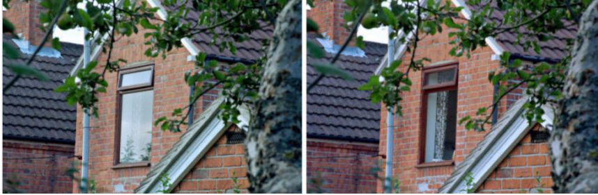
Figure 15.3: Because that TM and TE lights will be reflected differently, polarizer filter can produce remarkable effects on the quality of the photograph by reducing glare [104].
