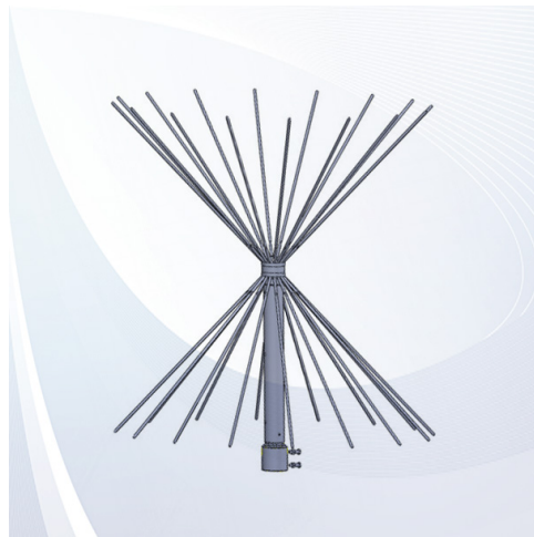
Figure 25.12: A bicone antenna can be thought of as a transmission line with gradually changing characteristic impedance. This enhances impedance matching and the radiation of the antenna (courtesy of antennasproduct.com).
