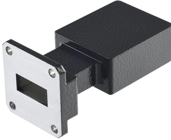
Figure 21.3: A rectangular waveguide terminated with a short at one end, and an open circuit at the other end. The open end can also act as an antenna as it also radiates (courtesy of RFcurrent.com).
