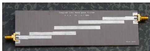
Figure 21.9: A microstrip filter designed using concatenated resonators. The connectors to the coax cable are the SMA (sub-miniature type A) connectors (courtesy of aginas.fe.up.pt).
