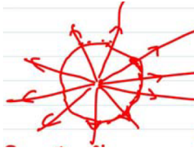
Figure 7: Electric flux from a point charge satisfies Gauss's law.
