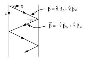
Since we define  $\beta_x = \beta \cos \theta$ ,  $\beta_z = \beta \sin \theta$ , the wave propagates in a direction making an angle  $\theta$  with the  $\hat{x}$ -direction. Since the guidance condition requires that  $\beta_x = \frac{m\pi}{b} = \beta \cos \theta$ , the plane wave can be guided only for discrete values of  $\theta$ .
