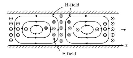
The sketch of the fields for  $TM_1$  and  $TE_1$  modes are as shown above. For the TM mode,  $H_z = 0$ , and  $E_z \neq 0$ , while for the TE mode,  $E_z = 0$ , and  $H_z \neq 0$ . Tangential electric field is zero on the plates while tangential magnetic field is not zero on the plates. The above is the instantaneous field plots.  $\mathbf{E} \times \mathbf{H}$  is in the direction of propagation of the waves.
