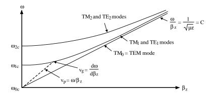
Since  $\beta_z = \frac{\omega}{c} \left[ 1 - \left( \frac{\omega_{mc}}{\omega} \right)^2 \right]^{\frac{1}{2}}$ , a plot of  $\omega$  versus  $\beta_z$  is as shown. When  $\beta_z \to 0$ , the group velocity becomes zero while the phase velocity approaches infinity. When  $\beta_z \to \infty$ , or  $\omega \to \infty$ , the group and phase velocities both approach the velocity of light in free-space which is the TEM wave velocity.
