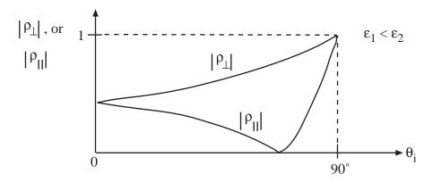
At normal incidence, i.e.,  $\theta_i = 0, \rho_{\perp} = \rho_{\parallel}$  since we cannot distinguish between perpendicular and parallel polarizations. When  $\theta_i = 90^{\circ}$ ,  $|\rho_{\perp}| = |\rho_{\parallel}| = 1$ . On the whole,  $|\rho_{\perp}| \geq |\rho_{\parallel}|$  for non-magnetic materials.
