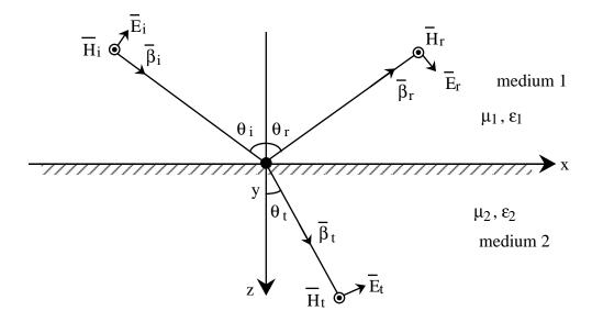
The magnetic field is polarized in the y direction, and they can be written as
