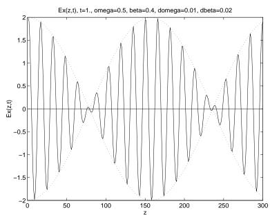
The first factor in (4) is rapidly varying while the second factor is slowly varying. The slowly varying term amplitude-modulates the rapidly varying term giving rise to the picture as shown.
