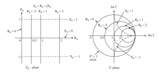
$Z_n$  is a complex number and can be represented by a point on the  $Z_n$ -plane, and  $\Gamma$  is a complex number and can be represented by a point on the complex  $\Gamma$  plane.
