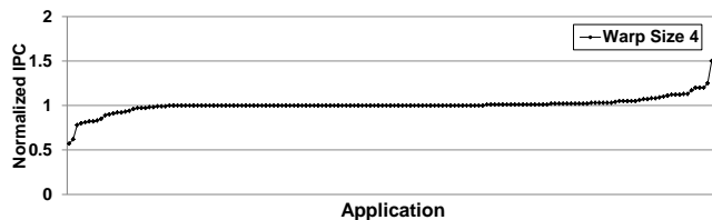
(a) Performance of 165 real world applications using a warp size of 4, normalized to a warp size of 32.
