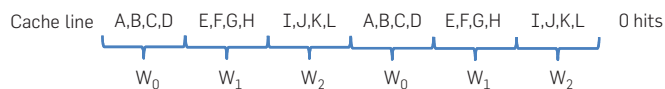
Figure 3. Example access pattern (represented as cache lines accessed) resulting from a throughput-oriented round-robin scheduler. The letters (A,B,C,...) represent cache lines accessed. W_i indicates which wavefront generated this set of accesses. For example, the first four accesses to cache lines A,B,C,D are generated by one instruction in wavefront 0.
