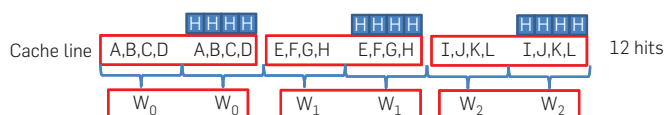
Figure 4. Example access pattern resulting from a hardware scheduler aware of its effect on the caching system. The red boxes highlight where scheduling improves locality by changing memory access order.
