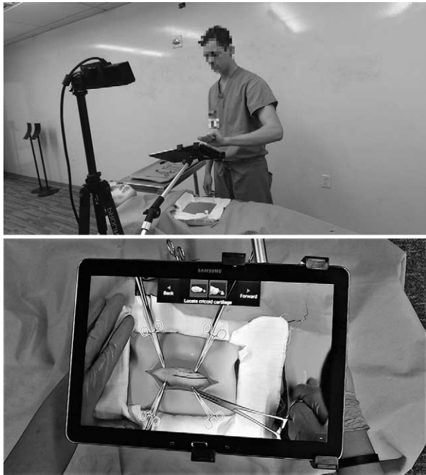
FIGURE 1. Top: STAR tablet-based setup. The tablet is held in place between the patient and the user with a mechanical bracket. Bottom: First-person view of an instruction received with the STAR tablet-based setup. The augmentation consists of 2D lines and images. The view of the camera is displayed on the device's screen.
