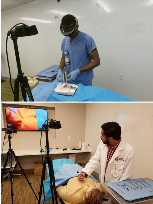
FIGURE 6. Experimental setup used to validate Augmented Reality Head-Mounted Displays (ARHMD) as surgical telementoring devices. Participants received surgical instruction from either the STAR ARHMD Trainee System (top) or a nearby monitor (bottom).
