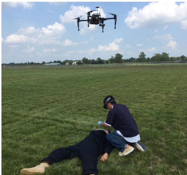
FIGURE 7. STAR's envisioned scenario for remote medical assistance in rural areas. A drone-mounted camera captures the view of the operating field, which will be sent to the remote specialist. The mentee located in the rural area will then receive surgical instructions from the specialist via the STAR Augmented Reality Head-Mounted Display.
