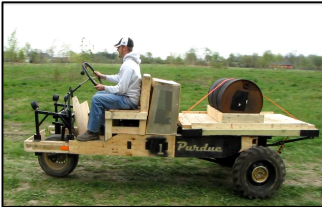
FIGURE 1a. Wood-frame/belt transmission BUW prototype constructed at Purdue (April, 2010)
