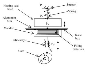
Figure 4. Ports of heating seal module
