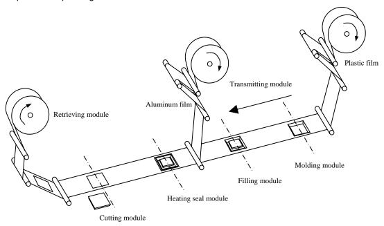
Figure 9. Plastic box packaging machine configuration
