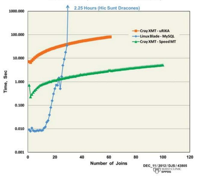
COMPUTATION RATES FOR MAXIMUM LIKELIHOOD GENOME ASSEMBLY ALGORITHM RUN ON CRAY XMT-2 AND INTEL-BASED SERVER WITH OPENMP (Algorithm Implemented Using MTGL Hash Tables and Array Data Structures; Cray XMT-2 System with 64 Processors and 2 TB RAM; Intel Xeon Server with 4 CPUs, 32 Cores, and 0.25 TB RAM)
