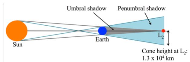
**Fig. 12.** Translation of Earth shadow avoidance requirement to maximum cone angle constraint.
