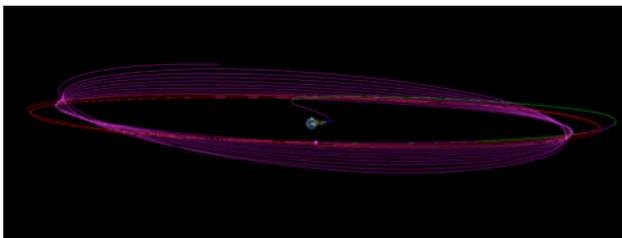
**Fig. 17.** Trajectory generated within ATD ephemeris (magenta) and STK (green and red) overlaid, as viewed looking down the Earth to  $L_2$  line.
