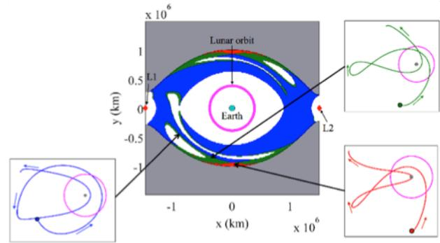
**Fig. 9.** Sample apoapsis map in the CR3BP for prograde initial conditions, with colored regions differentiating transfer geometries as illustrated via the inset images.
