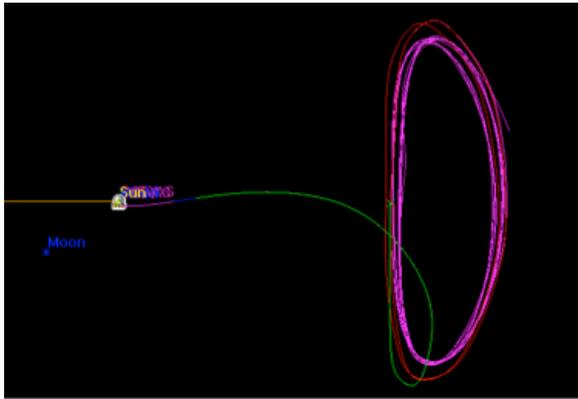
**Fig. 16.** Trajectory generated within ATD ephemeris (magenta) and STK (green and red), viewed in RLP frame.
