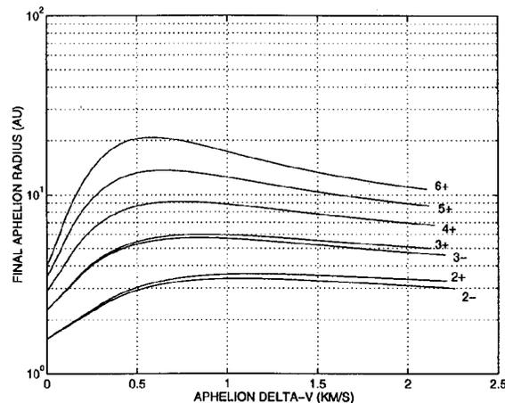
Fig. 2.  $\Delta V$ -VGA Performance Versus Aphelion  $\Delta V$ .
