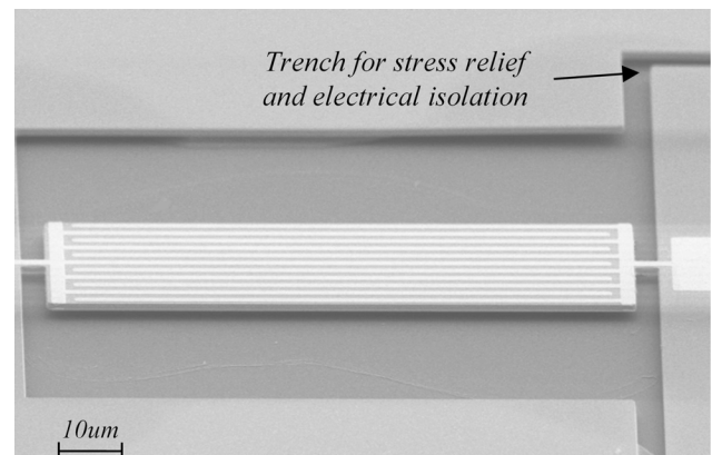
Figure 2: SEM of a 90um x 40um LN contour-mode resonator with 11 finger electrodes.
