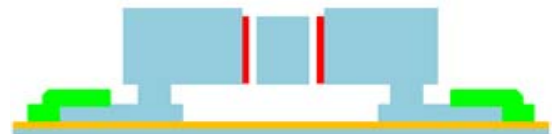
Figure 5. After Fig. 4h and metallization, hafnia + air gap devices are vapor HF released to achieve 10nm air gap.
