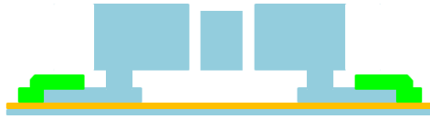
Figure 6. An additional wet etch to remove hafnia after the step in Fig. 5 resulted in 100nm air gap devices.
