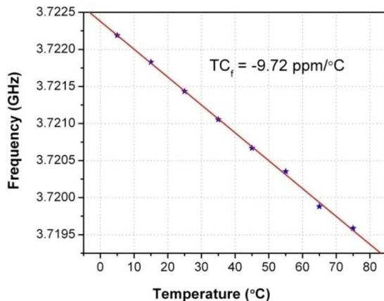
**Figure 6.** Resonant frequency as a function of temperature. This figure shows a linear dependence with a temperature coefficient of  $-9.72 \text{ ppm}/^\circ\text{C}$  over a temperature range of  $5 - 75^\circ\text{C}$ .
