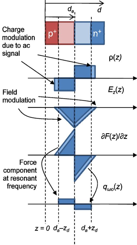
**Figure 2:** Illustration of principle of actuation in the input junction showing the charge density  $\rho$ , electric field in the thickness direction  $E_z$ , and force component at resonant frequency  $q_{\omega_0}$  throughout the structure.
