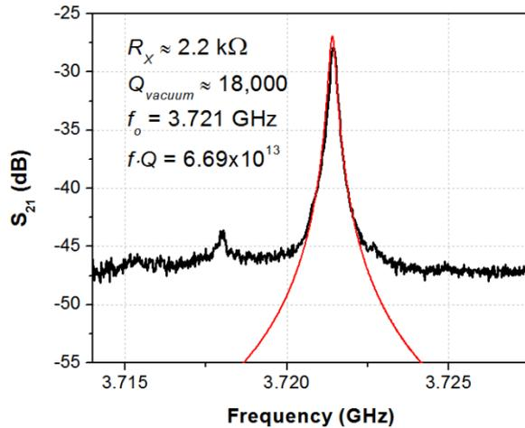
**Figure 5.** Pseudo-differential transmission magnitude plot of pn-diode resonator shown in Figure 1 in vacuum after SOT de-embedding demonstrating  $Q \sim 18,000$  at 3.72 GHz. Red trace shows fit with equivalent circuit model from (10)-(11). A bias voltage of  $-5V$  is applied to each junction.
