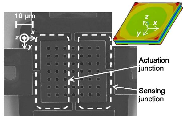
**Figure 1:** SEM of the  $40 \mu\text{m} \times 40 \mu\text{m}$  pn-diode transduced micromechanical resonator. The resonant frequency of 3.72 GHz is determined by the silicon device layer thickness (no electrodes or other mass loading layers). The thickness displacement amplitude of the resonant mode shape is shown in the inset plot. Etch holes are required for timed HF release.
