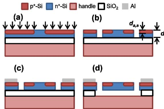
**Figure 3:** (a) The 1.3  $\mu\text{m}$  device layer of an SOI wafer is selectively doped using boron implantation and annealed to achieve the desired junction depth of 0.65  $\mu\text{m}$ . (b) The device layer is etched to define the resonator and pads. (c) Aluminum is deposited and etched to define the interconnect and pad structure. (d) The device layer is released via timed HF etch.
