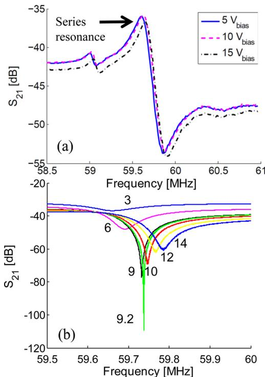
FIG. 2. (Color online) (a) Forward transmission coefficient,  $S_{21}$ , of the type-II, high isolation and (b) type-I devices under varying DC bias conditions ( $V_{bias}$ ) on both the input and output ports.
