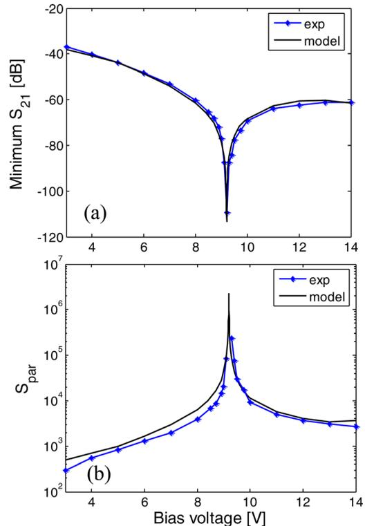
FIG. 3. (Color online) (a) The modeled and extracted minimum  $S_{21}$  from Fig. 2(b) and (b) the associated sharpness of the parallel resonance frequency response as defined by Eq. (2).
