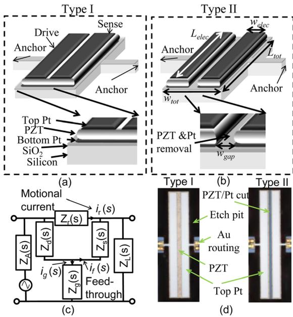
FIG. 1. (Color online) Illustrations of the two fabricated device types: (a) type-I without and (b) type-II with removed PZT and common Pt electrode. (c) Equivalent circuit of the type-I device with source and load impedances and labeled motional current,  $i_r(s)$ , due to the electromechanical resonator and feed-through current,  $i_f(s)$ . (d) Top view of the fabricated devices.
