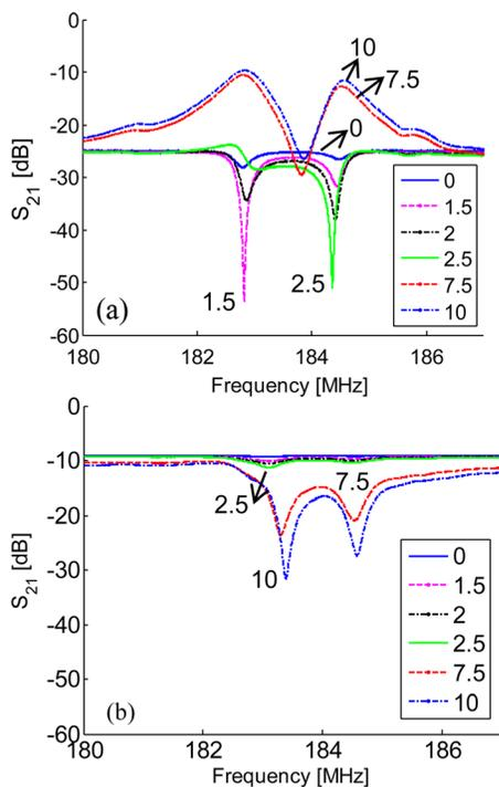
FIG. 4. (Color online) The frequency response of the type-I higher order modes with (a)  $Z_g = 1.65 \Omega$  and (b)  $Z_g = 15 \Omega$  revealing the impact of the finite resistance to ground on the response.
