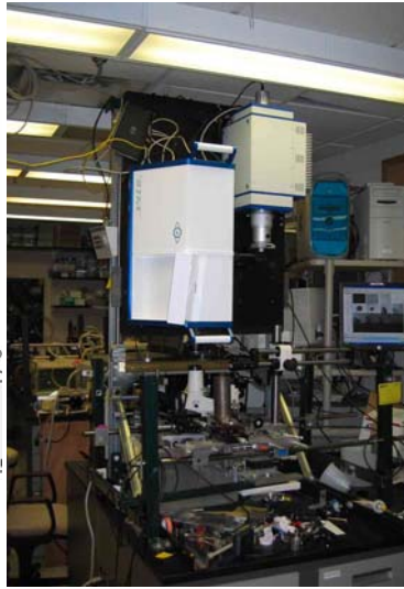
Figure 1. Experimental setup of the ultra high-speed imaging system (schematic on left, photo on right). The full frame camera is coupled to the streak camera on a vertical optical table. Below is a hybrid microscope with a 40x water immersion long distance objective. Droplets are positioned in the acoustic and optical field using a polyethylene tube (shown in cross-section).
