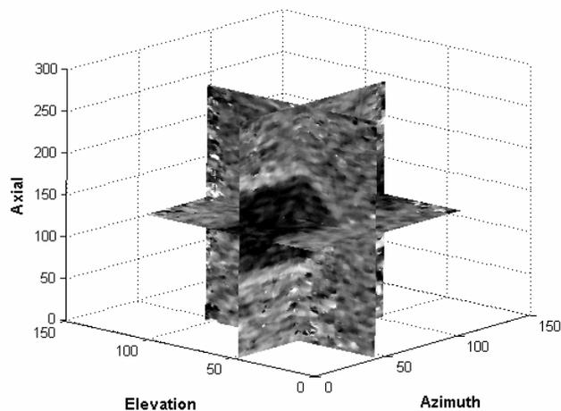
Figure 4. Perpendicular slices of the 9 mm cylindrical inclusion phantom 3-D strain image generated using 3-D beamforming and 3-D displacement estimation. The transducer is located at the bottom of the image.
