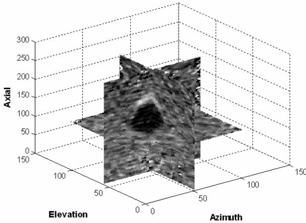
Figure 6. Perpendicular slices of the 9 mm spherical inclusion phantom 3-D axial strain image generated using 3-D beamforming and 3-D displacement estimation. The transducer is located at the bottom of the image.
