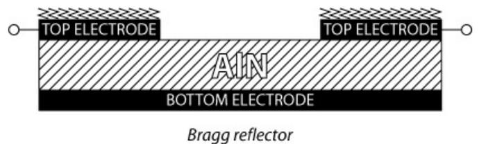
Figure 1. Schematic cross section of the resonators loaded with an organic layer.
